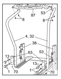
are at the same height. Do not tighten the Handrail Knobs yet. Always attach each Handrail with two Handrail Knobs. Attach the Console Base (87) (see assembly step 5 on page 6). Insert a Handrail Plug (70) into the unused hole in each Handrail (4, 32).
